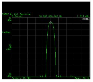
Figure 5-2 10 MHz Reference Clock Accuracy Test
