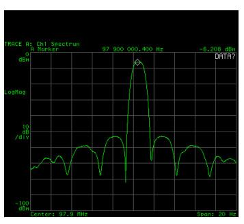
Figure 5-1 Center Frequency Accuracy Test
